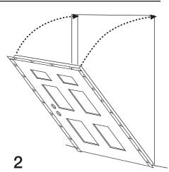
Tip complete pre-hung unit into opening, making sure it will swing the correct direction.
