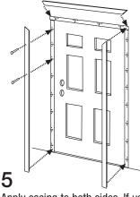
Apply casing to both sides. If using wood, pre-cut the pieces. Mark the location of the oval slots on each piece and fasten to the wall with the nail or screw going through the oval slot and into the framing material. If using
