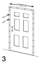
Check margins between door and frame. Center in rough opening left to right. Level header by shimming under the threshold or the frame. Check for proper alignment and fasten with screws or nails in the holes provided. Remove pre-hang clip.
