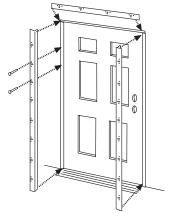
Slide the outer L-shaped pieces (See Detail 4A) into the inner section already on the wall. Start with the header first insuring header is centered over the jamb legs and then insert outer pieces into each jamb leg. Make sure outer jamb pieces are tight to the outer head piece. Ensure each of the three pieces are snug to the wall before fastening with screws or nails in the holes provided.
